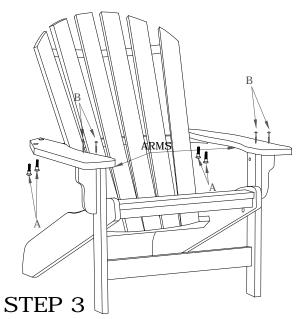
Attach Arms to front Legs from the top using screws (B). Bolt Arm Assemblies to Back Assembly using Bolts (A) as shown.
