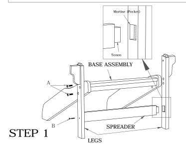
Attach Spreader tenon into mortise (pocket) on Leg Assemblies and attach with screws (B) as shown. Bolt legs to Base Assembly using bolts (A).
