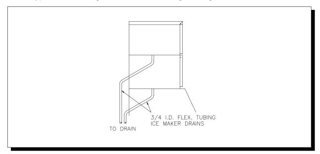
11. Electrical, water and drain locations are shown on the following drawing: All dimensions are in inches.
