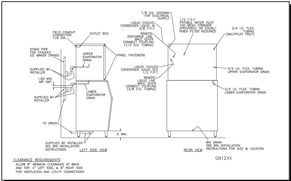
2. Level the bin with adjusters on legs, or by shimming if the bin is to be sealed to the floor. If gaps due to shims are greater than 1/8 inch, install a cove molding around the bin bottom. Seal the bin or molding to the floor with NSF Certified RTV sealant (Dow-Corning RTV 732 or equal).
