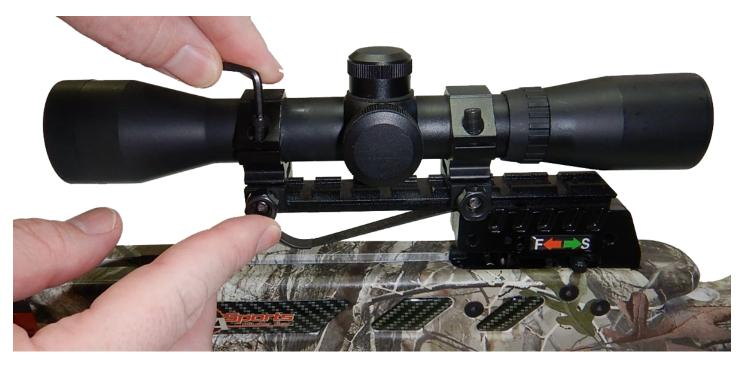
Realign the crosshairs or reticules to vertical tighten the upper rings.
