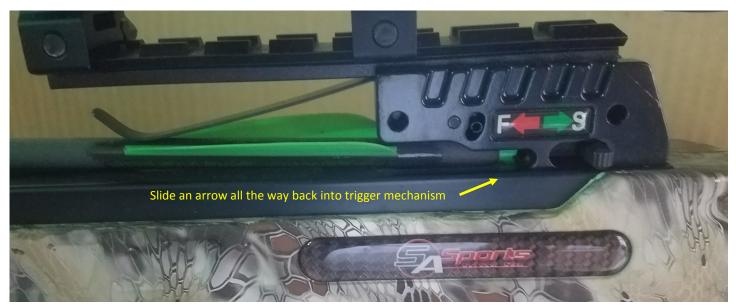
You will now be able to switch the safety to the fire position. Push the safety switch to the FIRE position and LEAVE IT ALONE in the Fire position. The safety will engage when you cock the bow. Simply remove the arrow and your bow will be ready to cock.
