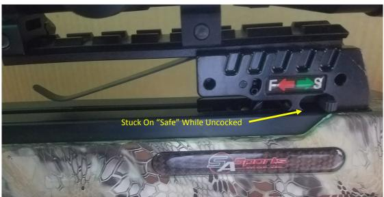
Insert an arrow into the trigger mechanism sliding it all the way back ,while the bow is uncocked as shown below. This will engage the anti dry-fire mechanism.
