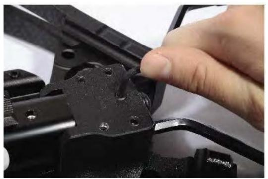
6. Insert the (7) foot stirrup into the two holes on the front of the (2) riser. Make sure the 2 notches in the foot stirrup are facing towards the (12) grub screws used to secure the foot stirrup, tighten securely.
