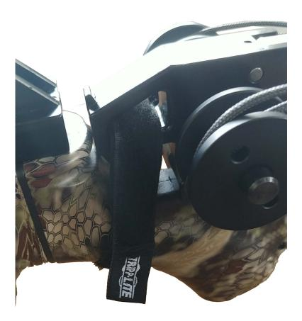
Note: If you are unable to hold the crank device down in place while cranking to avoid pulling the crank device out of the port and damaging the stem (Not Warranty) then you will need to use a piece of Velcro(tm) or hook and loop strip as shown in order to secure it in place while cranking. Make sure it is tight and secure so that your cranking motion does not pull the device from the crossbow.
