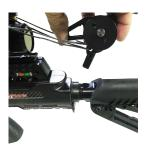
3. Place the Post on the crank device into the receiving port hole on the stock. The post is angled and must be positioned with the post toward the assembly/scope/ trigger front of bow. The hole (pictured at left) is located just behind the trigger assembly and scope eye piece. Be sure your adjustable rear stock is in the first positive click position so that the hole is free from obstruction. USE **VELCRO IF REQUIRED -**SEE PICS PG 5
