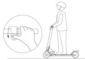
Step 3: When the scooter starts to coast, put both feet on the deck and press the accelerator (Throttle). The accelerator initiates once the coasting speed exceeds 5km/h.
