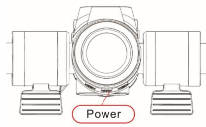
Press and hold the POWER button to turn on the display.
