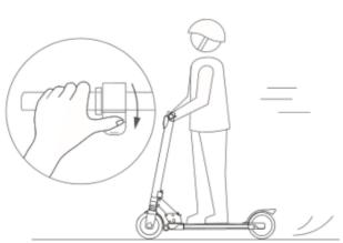
Step 4: Release the accelerator and the kinetic energy recovery system (KERS) initiates automatically to brake slowly; and squeeze the brake lever for a suddden brake.
