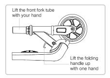
Lift the folding handle up with one hand and lift the front fork tube with the otherhand, and hear a "click".
