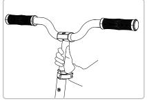
Press the adjustment marble with one hand and adjust the telescopic rods to the proper position with the other hand.
