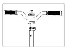
Use the screwdriver to lock the handle block.
