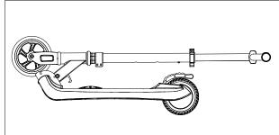
Lift the folding handle in one hand and gently pull the standpipe back with the other hand when hear the "click" to complete the folding.
