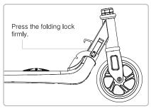
Press the folding lock firmly. (the folding lock can adjust the tightness)
