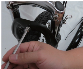
Loosen pre-installed screws on front fork
