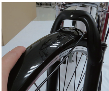
Installation of the fender
