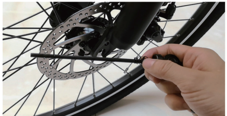
Installation of the front axle Installation of the spring
