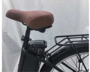
Lock the seat tube clip
