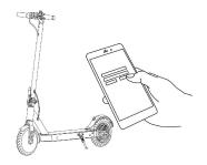
2.Power on the Gyrocopters Flash Pro Max,then open the APP,it will automatically search for Bluetooth devices.
