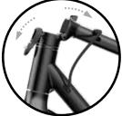
Release folding clip to fold steering column
