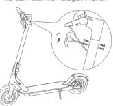
2. Attach the handlebar to the stem
