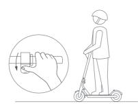
When the scooter starts to coast, put both feet on the deck and press the accelerator (the accelerator initiates once the coasting speed exceeds 5 km/h)
