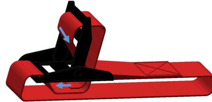
6. Insert the strap through the inner slot of the base.
