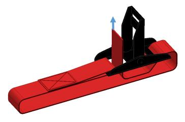
4. Insert the strap through the top slot of the handle.
