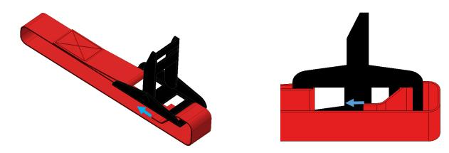
3. Feed the strap through the larger slot of the buckle on the opposite end.
