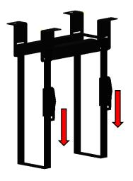
\*With the buckle in the open position, pull the straps from below the buckle to loosen.
