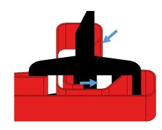
7. Pull the end of the strap to remove slack.
