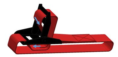
6. Insert the strap through the inner slot of the base.
