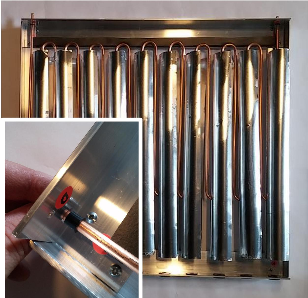
5) Slide plastic sleeves as far up as they can go through the hole in the frame. This is a general reference point for where the manifold will be positioned when assembly is complete.
