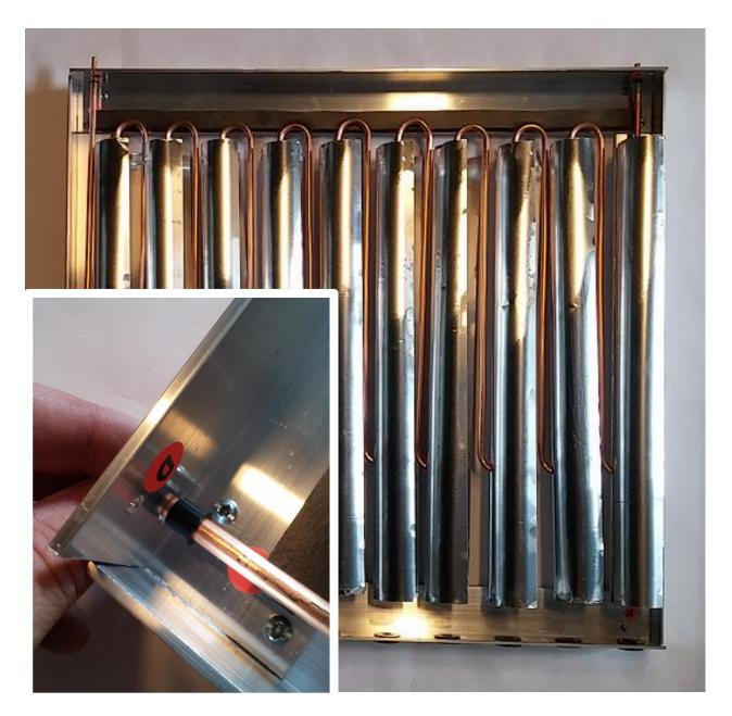
5) Slide plastic sleeves as far up as they can go through the hole in the frame. This is a general reference point for where the manifold will be positioned when assembly is complete. 6) Gently pinching the silver fins, slide a glass vacuum tube onto each of the 10 manifold sections (Figures 1, 2 & 3). Position pointy ends of tubes loosely in the plastic fittings (Figure 4).
