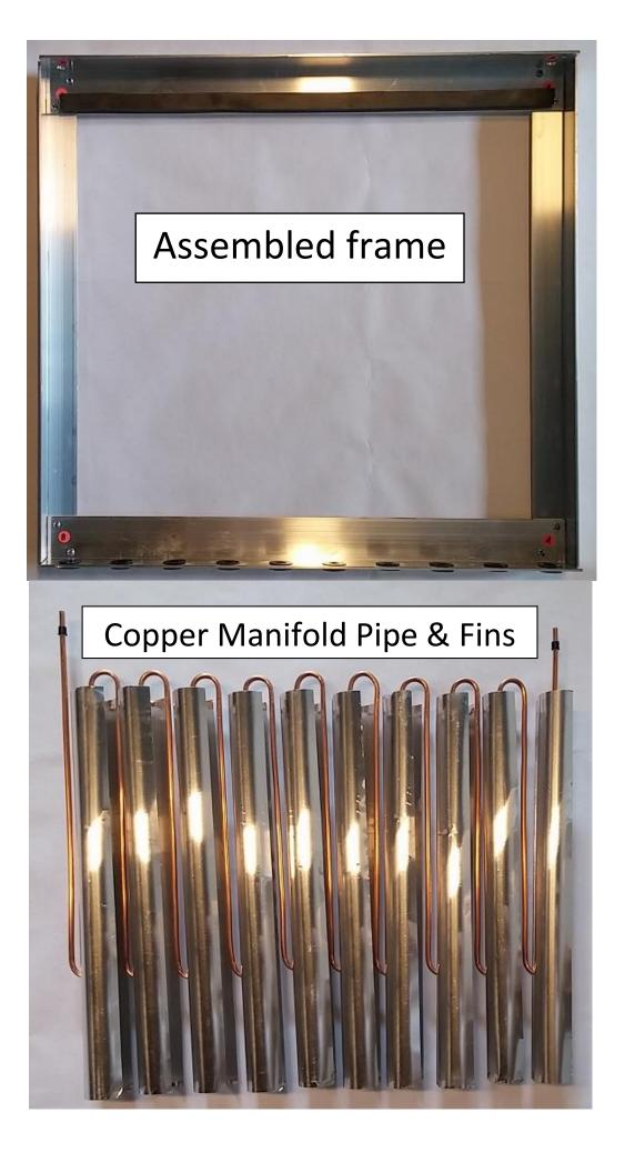
4) Slide ends of copper manifold pipe through the two holes in top face of frame. Position manifold where top curves of the copper pipe sit aligned with center of foam strip.
