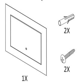
3.Mark a desired height of the mirror. Drill the required holes and insert the wall plugs. Note: Wall plugs supplied are only suitable for solid stone/brick walls. Please ensure the screws are fully tight.
