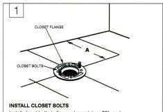
Install closet bolts in flange channel, turn 90°, and slide into place 6" (152 mm) apart and parallel to wall.
