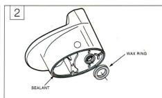
Invert toilet on floor (cushion to prevent damage), and install wax ring evenly around waste flange (horn), with tapered end of ring facing toilet. Apply a thin bead of sealant around toilet base.
