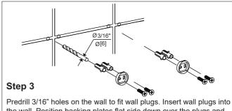
the wall. Position backing plates flat side down over the plugs and install screws.
