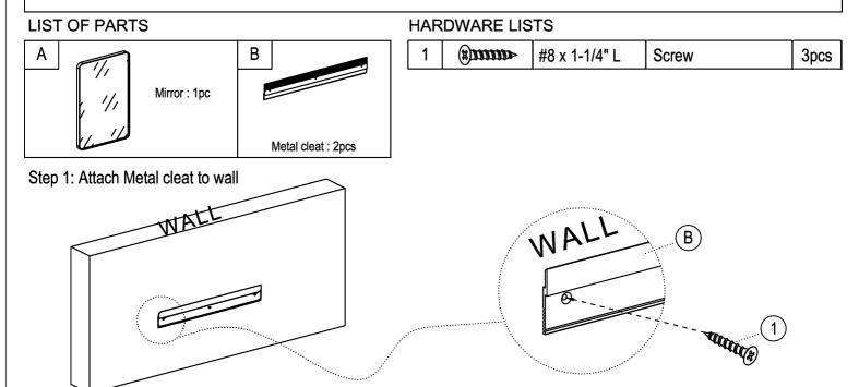
Based on the position of the metal cleat on the wall relative to the mirror to locate the mirror on the wall.
