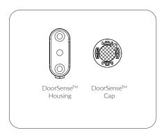
Remove magnet from housing and place DoorSense<sup>™</sup> Cap onto the magnet
