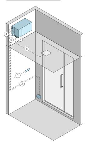
Connection between Nuvola Smart Power and the control panel
