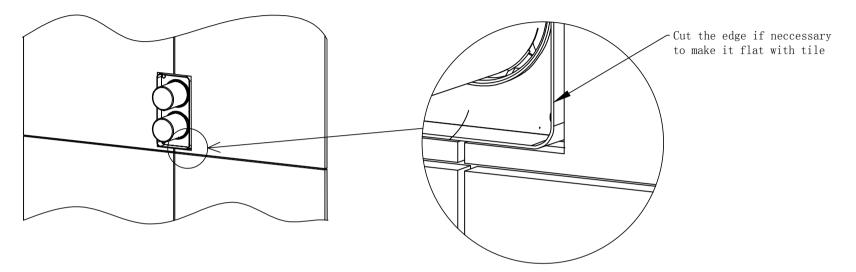
6. Remove protective caps. Install trim plate and handles.
