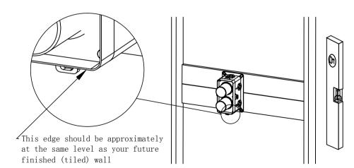
3.Use 1/2'' NPT fittings and thread seal tape for all pipe work according to the diagram below. No soldering close to the mixer body!
