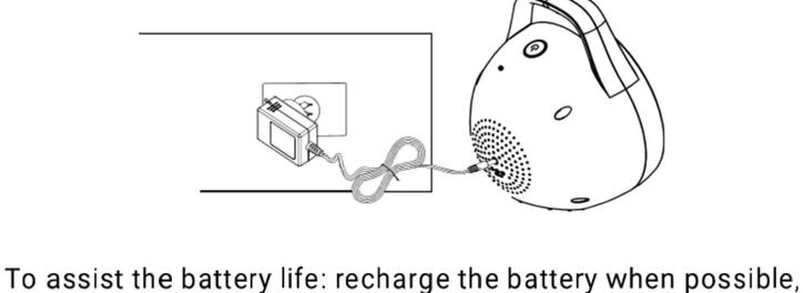
even after each use. Never let the battery run flat. Turn the pump off when not in use.
