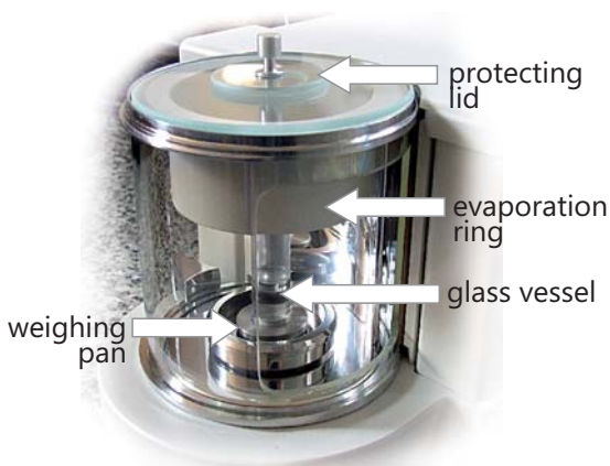
MYA 21.4Y.P (control of piston pipettes volume)
