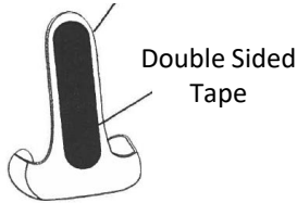
Install Tape on Backside of Remote Control Holder
