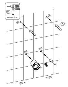
Drill the holes according to the marked points (the holes' depth must be deeper than the length of the expansion nut, the diameter shown as in the picture) and press the corresponding expansion nut into the hole.
