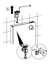
Take out the inlet valve upwards
