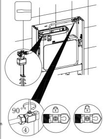
Open the stop valve on the hose to see whether it works and water runs into cistern tank
