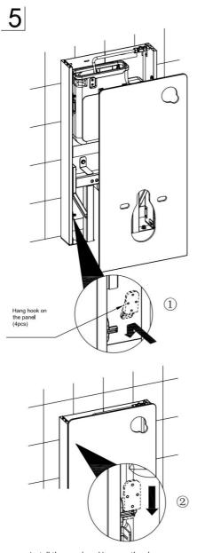
Install the panel, making sure the glass panel is carefully pushed close to the aluminium frame, then push the panel down until it is fully mounted on the hangers/hooks on the frame
