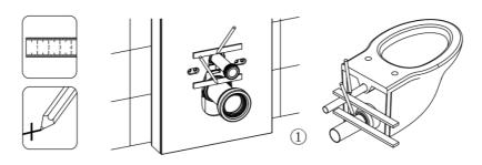
Mark on the straight flush pipe and drainage pipe
