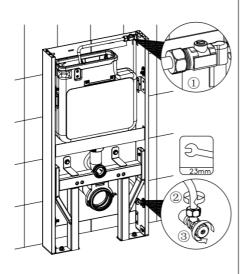
Click/mount the hose in to the holder bracket, then connect the hose into the valve
