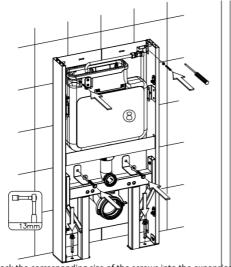
Lock the corresponding size of the screws into the expansion nut in the wall and steel expansion bolt on the floor
