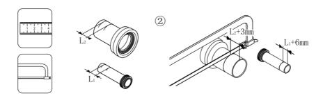
Cut the flush pipe and drainage pipe
