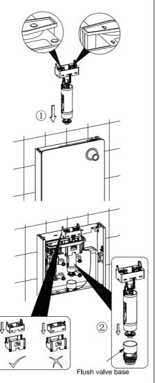
Install the flush valve downwards into the cistern body (Remark: make sure the flush valve bottom is aligned with flush valve base. And please make sure flush valve is installed in the shown direction during installation.
