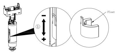
Adjust the float upwards to reduce the flush volume; or downwards to increase the volume.
