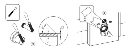
Use a file to chamfer the edge of the flush pipe and waste pipe
