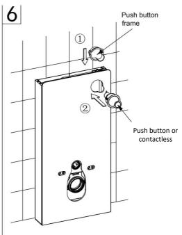
Install the push button frame and button onto the glass
