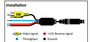
**Note:** If the camera is powered by reverse gear lamp signal, we recommend to install a relay between the power supply of the reverse signal and the power supply of the camera, to ensure a stable and uninterrupted power supply and to avoid unwanted errors in the vehicle computer.
