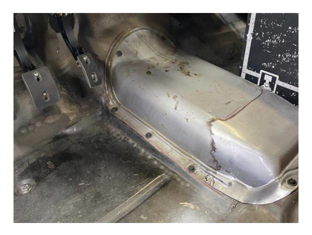
Set your new high hump cover down on the floor and mark the outside diameter as well as the hole locations. Once you have made your mark, you will be able to drill holes and make your final clean cut on the floor.
