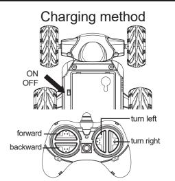
The RC car turn on , then the controler then on , controler's LED twinkle , when LED off , can start control.
