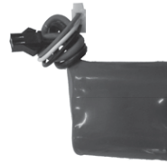
1100mAh 7.4v LiPo BATTERY
