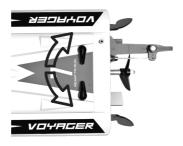
1. Twist the two cabin switches left or right. Then lift upward to open the cabin cover.
