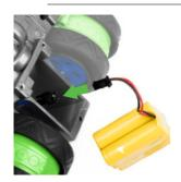
**3.** Plug in battery. Please note: Battery should be installed as illustrated below.
