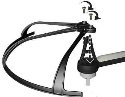
SCREW IN PROPELLER GUARD
