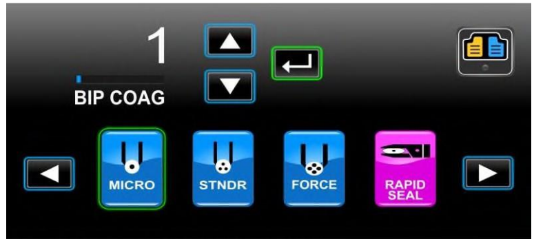
Mode: Micro - Low Intensity bipolar coag for delicate tissue.
