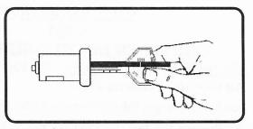
pointing upward on the door and deck locks, you will be reading the wafers in the space positions of 1, 3, 5, and 7. If the trap slot is pointing downward on the door and deck locks, you will be reading wafers in the space positions of 2, 4, and 6.
