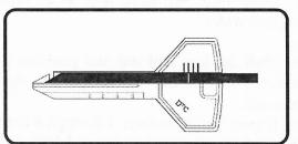
Remember that the door, deck and ignition locks are double-sided. You will trap and read one side and then turn the tool over and read the other side.
