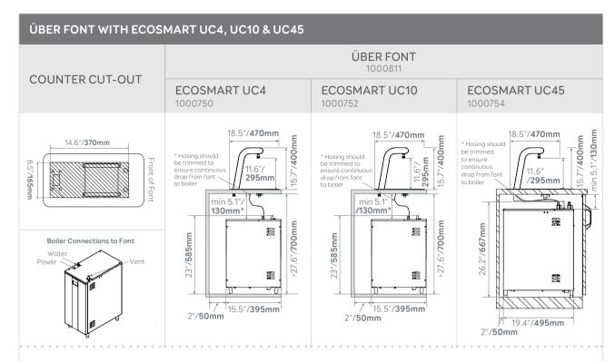
50mm/1.9" clearance required at each side and back of machine if installed in an enclosed cabinet.
