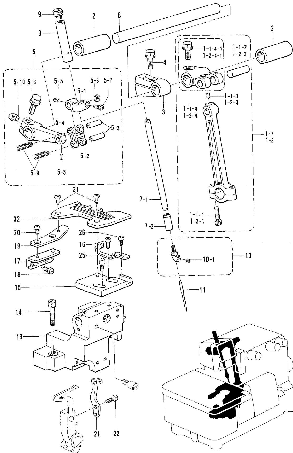
C. 針棒関係 /Needle bar mechanism/Nadelstangenvorrichtung/
