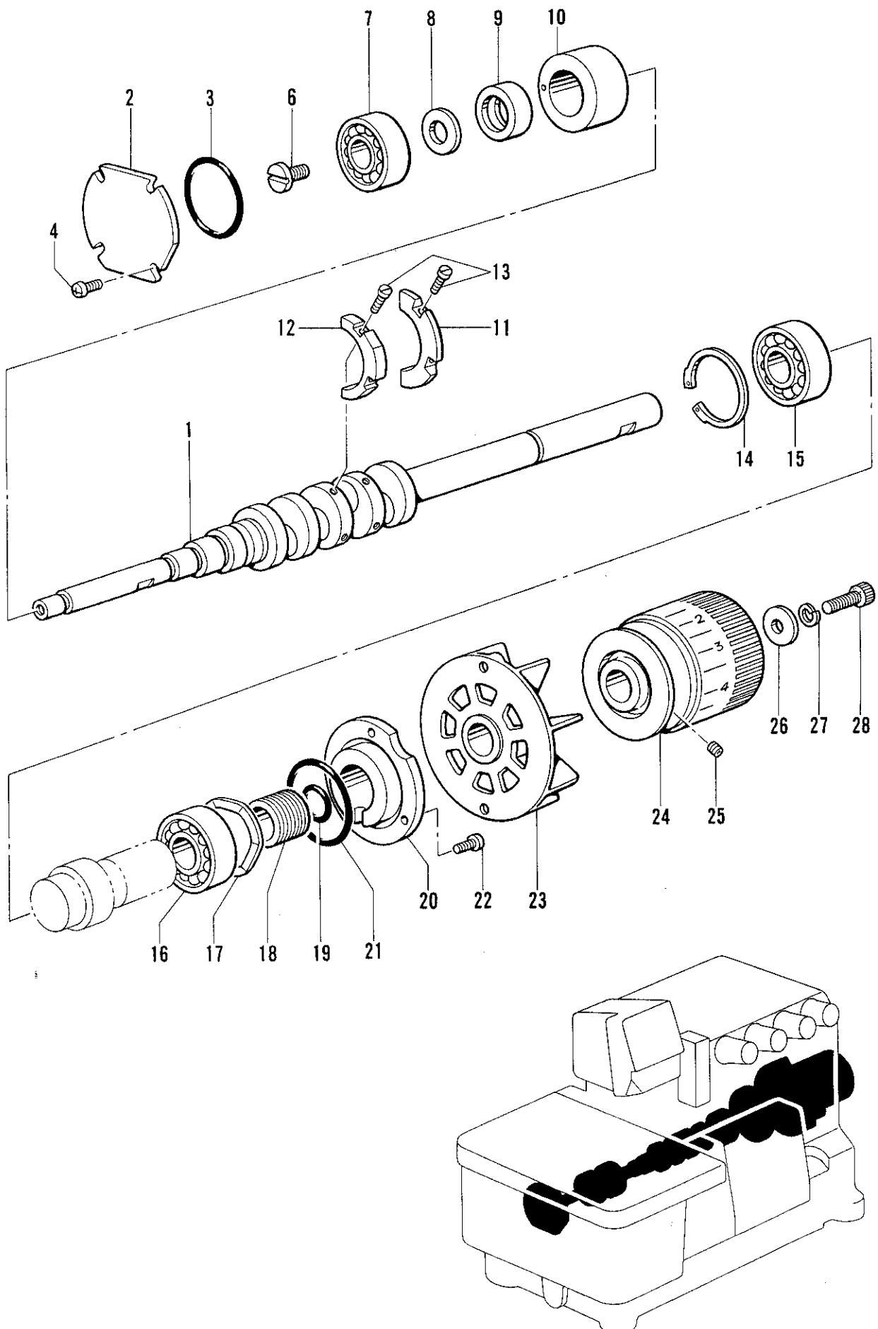
B. 駆動軸関係/Crank shaft mechanism/Kurbelwelle/
