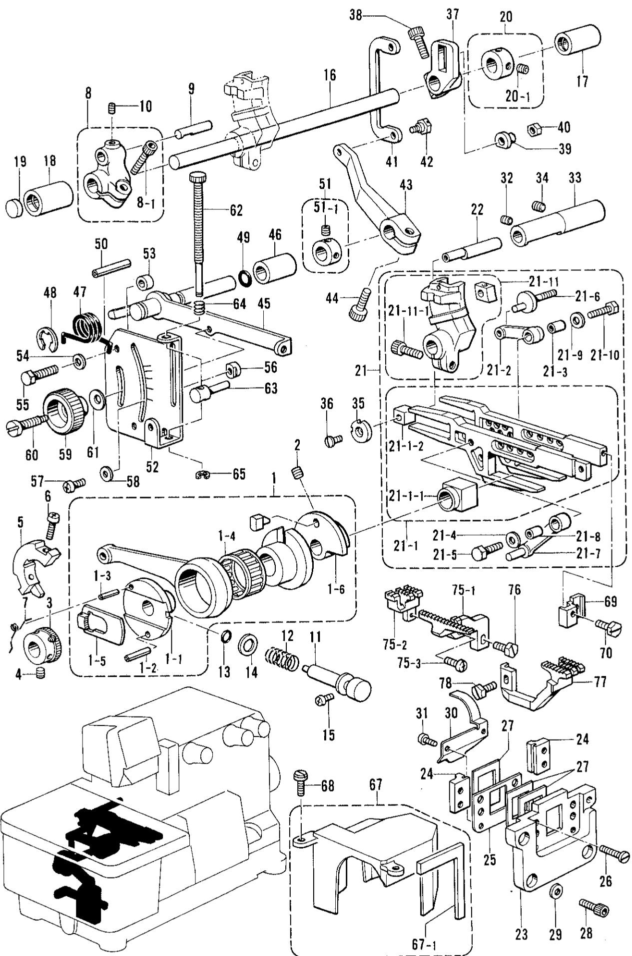
E. 送り関係/Feed mechanism/Transportvorrichtung/
