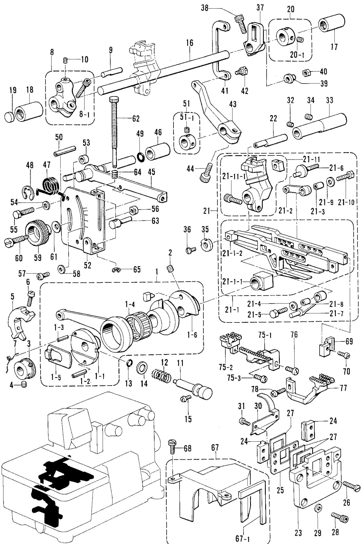
E. 送り関係/Feed mechanism/Transportvorrichtung/
