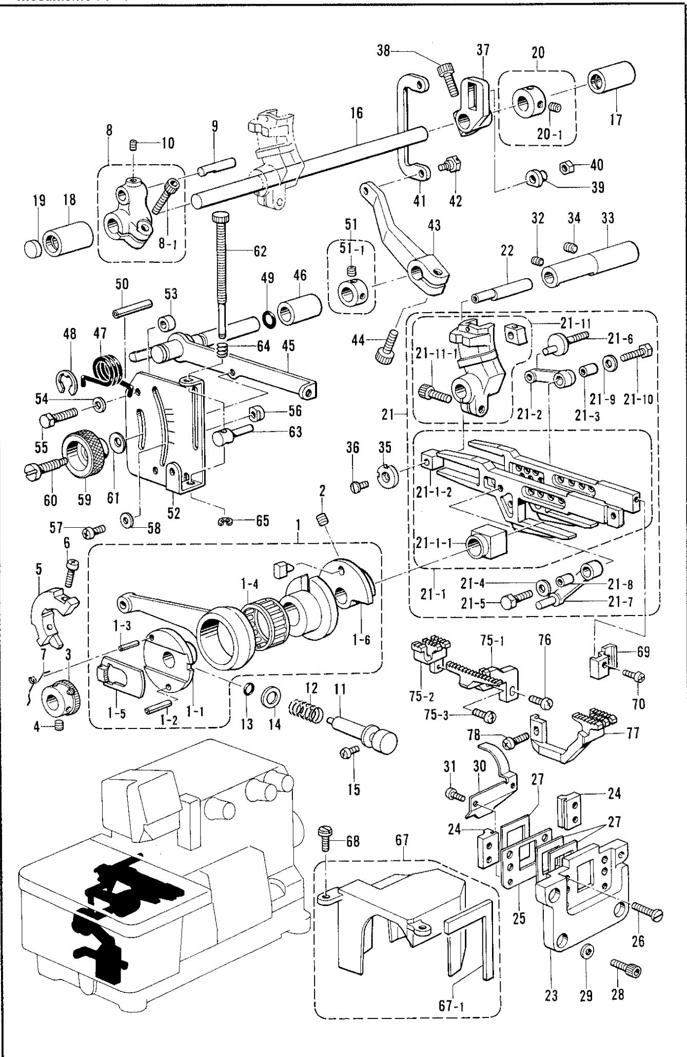
E. 送り関係 /Feed mechanism/Transportvorrichtung/
