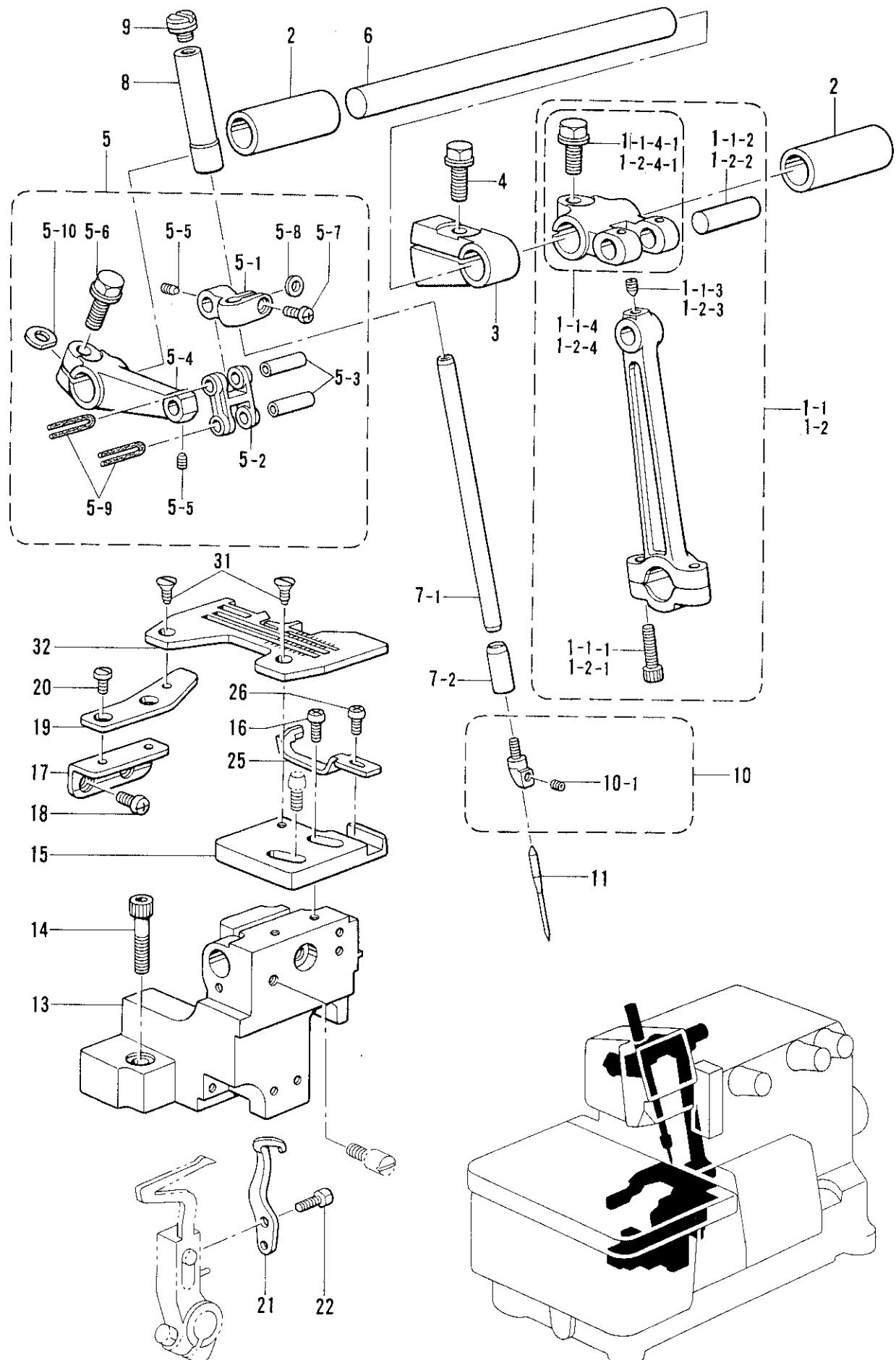
C. 針棒関係 /Needle bar mechanism/Nadelstangenvorrichtung/
