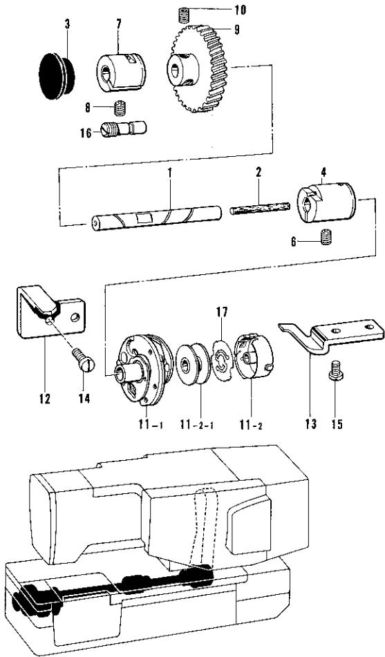
**R. Lower shaft mechanism**
