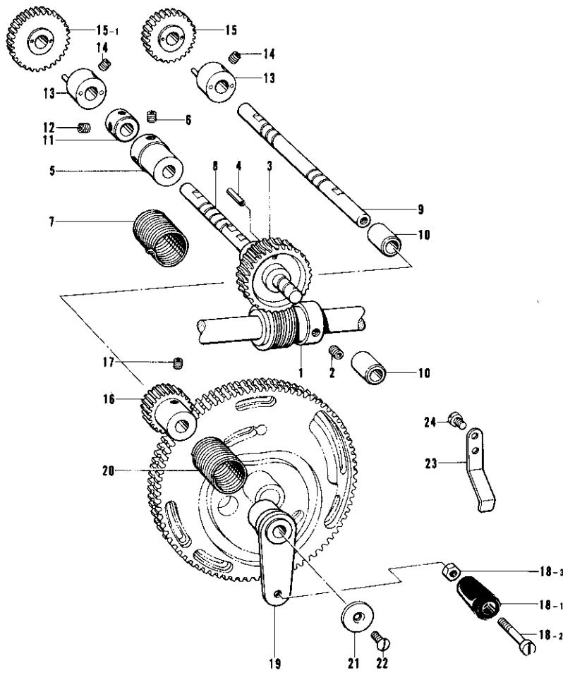
**N. Thread breakage detector**
