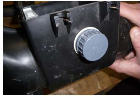
Fig. 3: Lateral sludge pump connection with stopper
