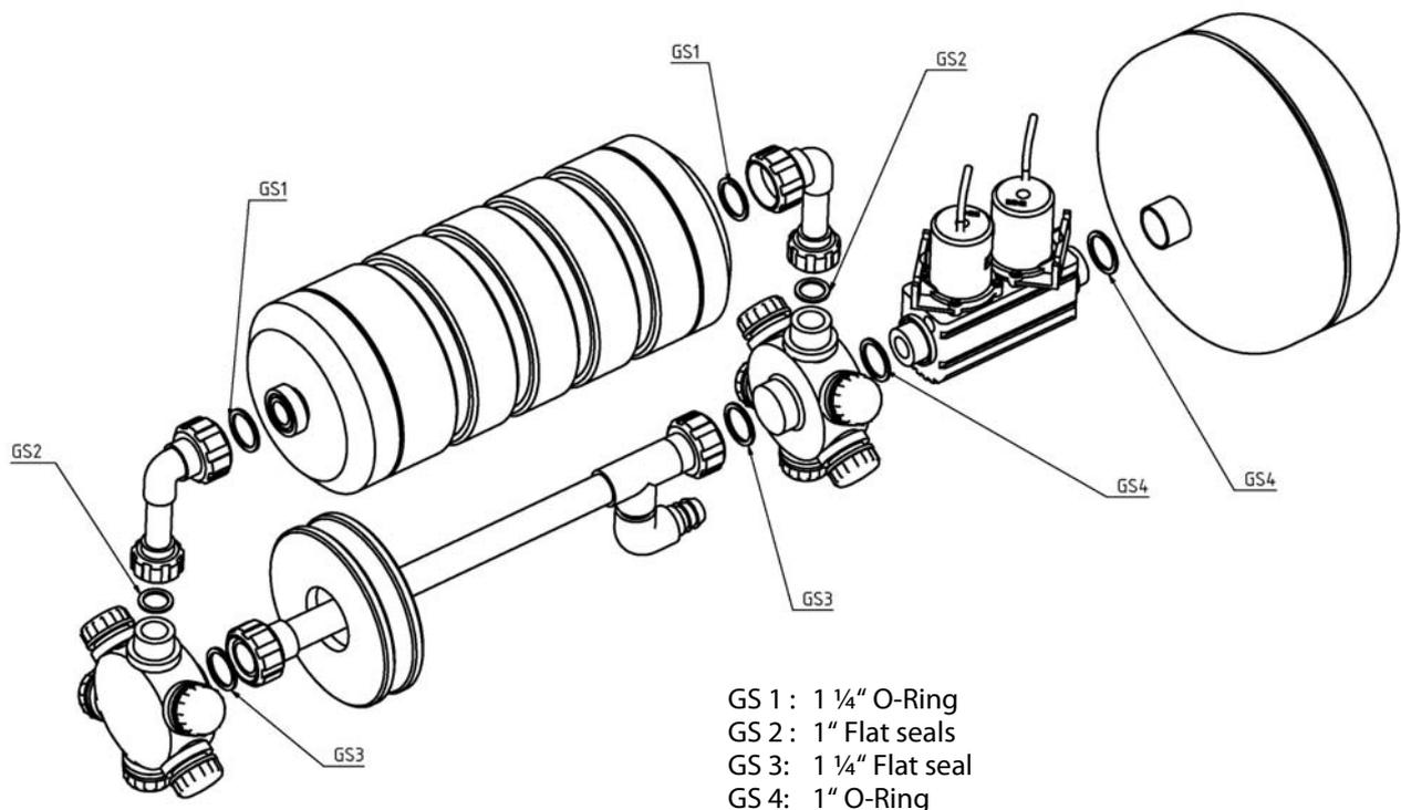
Fig: Layout of the membrane station
