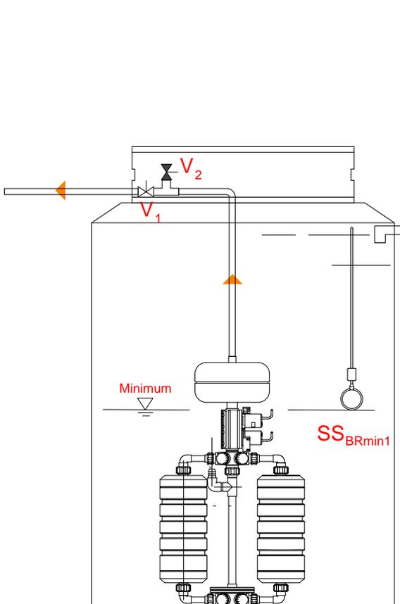
Cleaning device: normal filtration working
