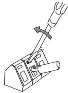
*Fig.: Operating mode spring terminal*
