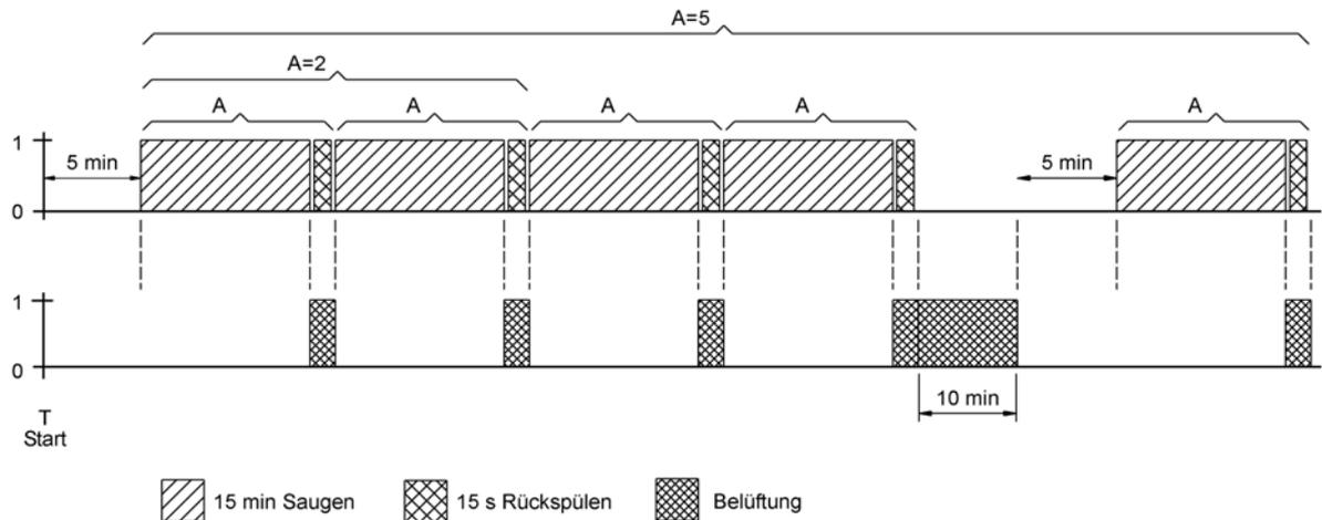
Fig.: Example of a pump cycle with  $A = 5$
