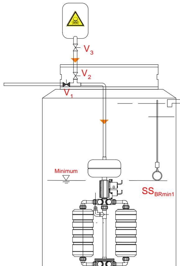
Cleaning device with connected canister (chem. fluid)
