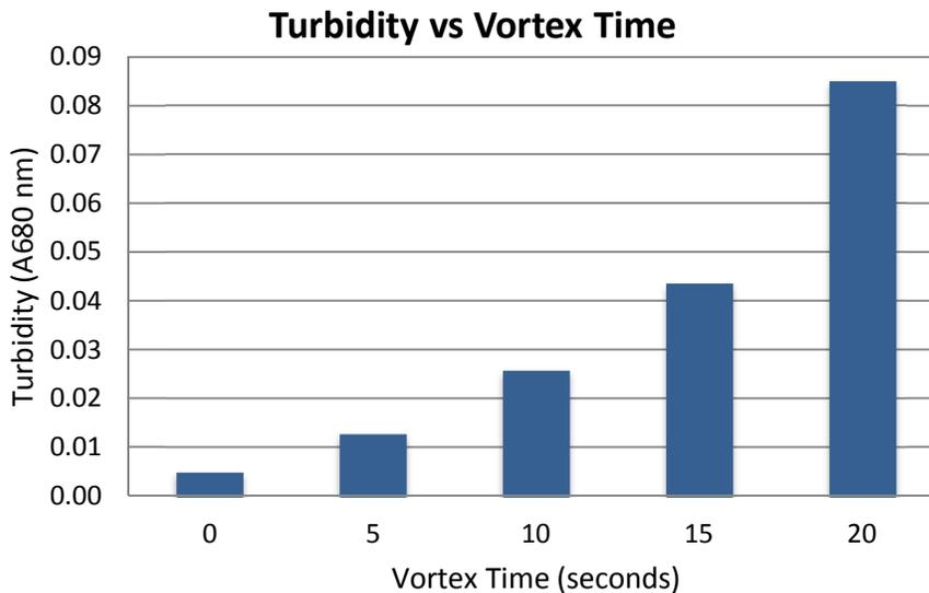
Aggregation was estimated by turbidity, measured by absorbance at 680 nm. The 30 second time point is off scale and not shown.
