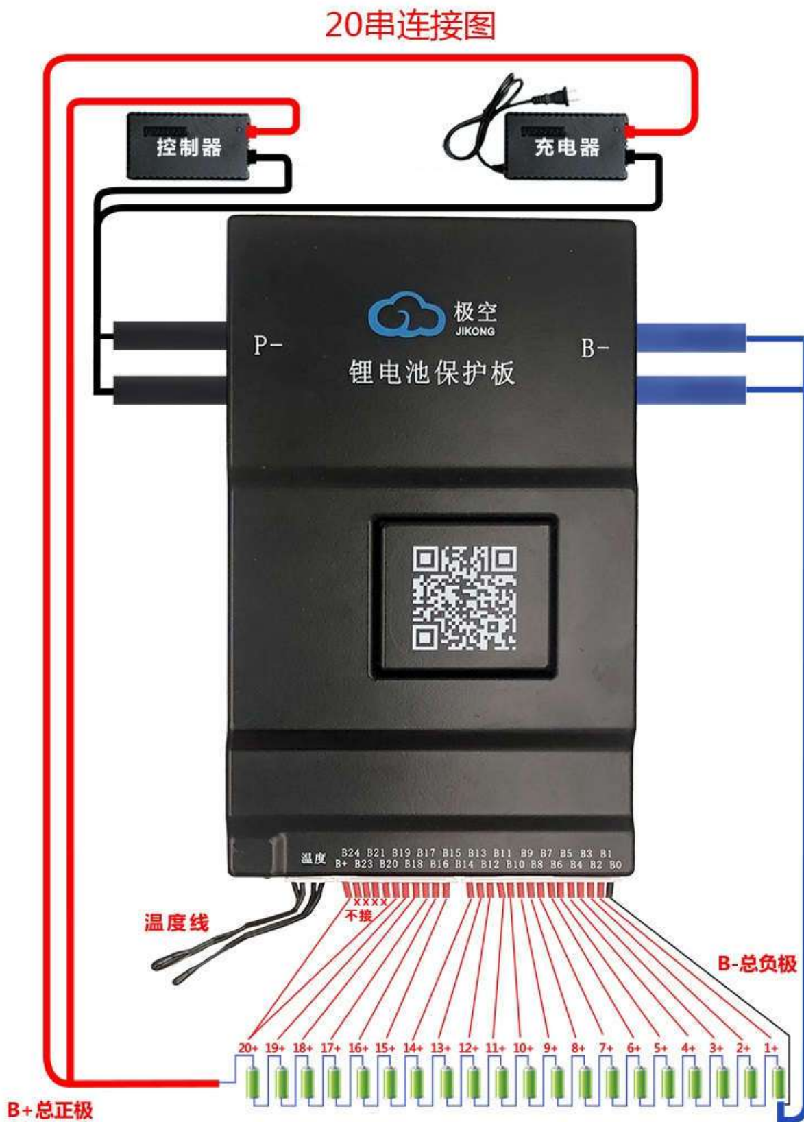
Figure 9 Diagram of 20 series battery connection
