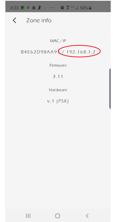
If IP address displays in format (xxx.xxx.x.x), you are connected to LAN. If not displayed, then see instructions on next page.
