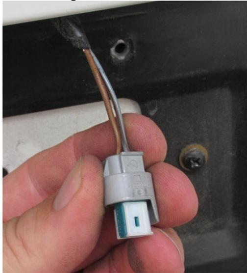
Now you can connect the new LED License Plate Bulb assemblies. Align the metal spring on the new lights the same orientation as the original lights you removed. Dock the 2 hard plastic tabs into the bumper first, then push up and clip in the side with the metal spring clip. Perform function test, and enjoy the look of your new lights!
