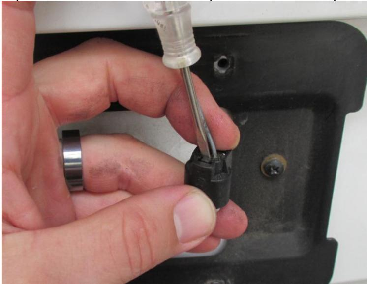
Under the outer connector shell, there is another locking shell, which is white. You need to pry underneath it and move it sideways to access the wire pin locks. Here is the locking shell in the locked position:
