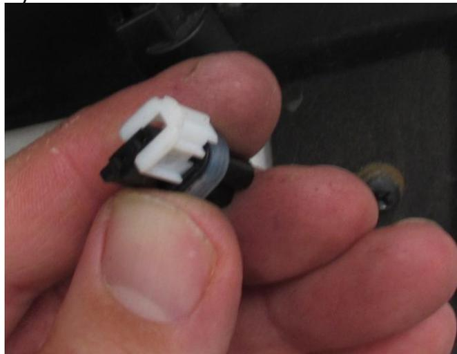
Once both the outer and inner connector shells are removed, you will find 2 windows on the connector to the wire pins. Inside these windows, there are small tabs on each wire pin. When you press down on them, the wire pins will be free to move and can come out of the connector.
