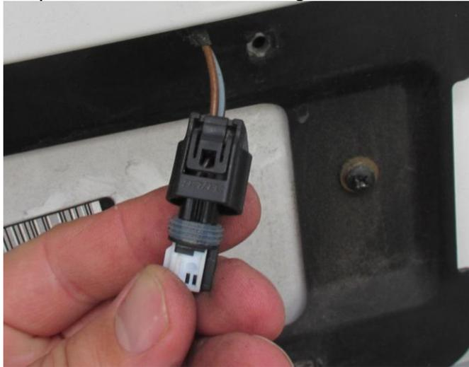
This is the shell moved to the unlocked position. Once unlocked, you can slide the white shell all the way off the connector and remove it completely.
