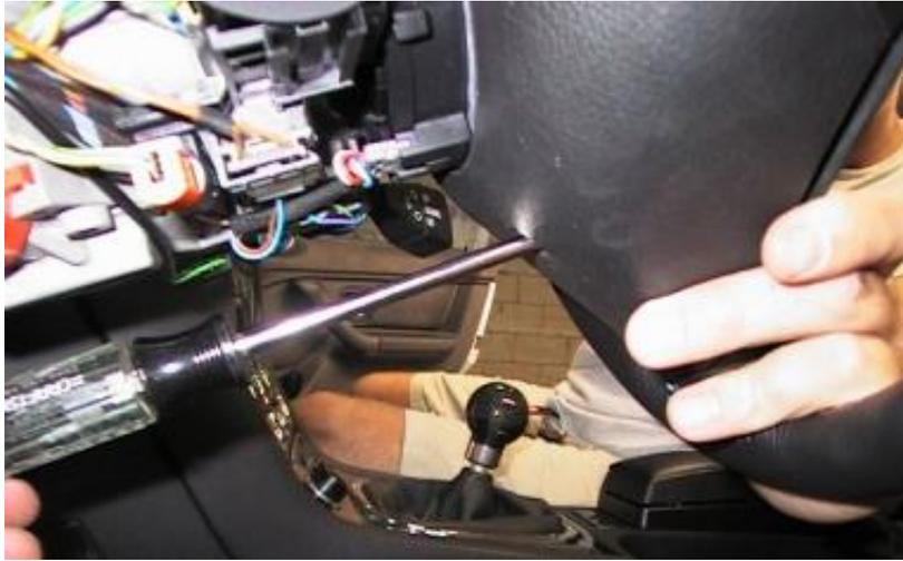
Figure 2. Removal of T30 Torx screw (1 of 2).
