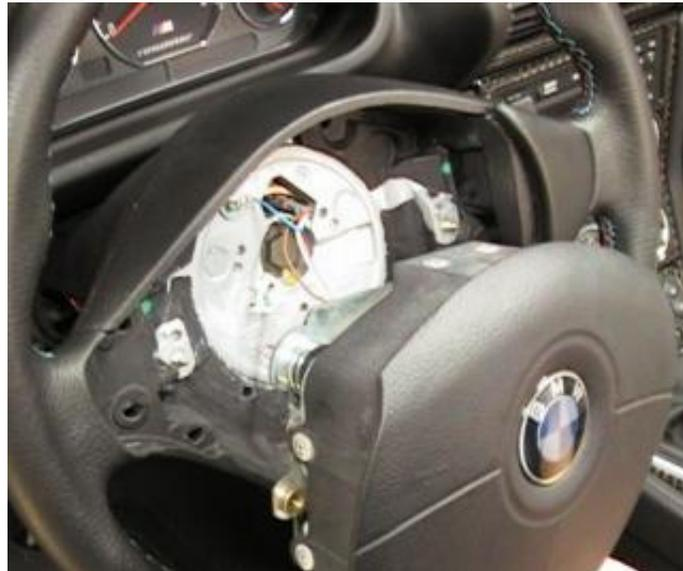
6. Pry out each of the 2 plastic Steering Wheel Tabs. See figure 4. It helps if someone can hold the airbag for you while you do this. You should be able to do it without any tools.
