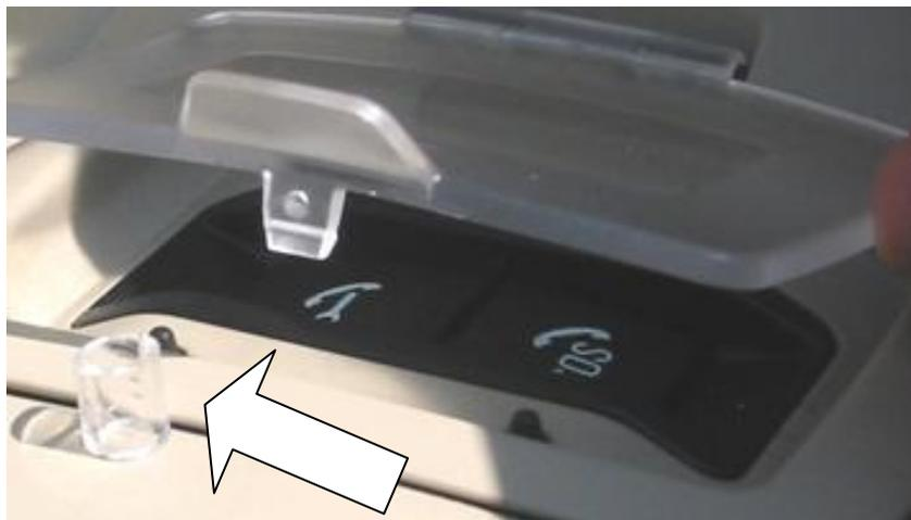
BMW Assist cover open showing "tab" and clear plastic tube (at arrow) ready for installation.
