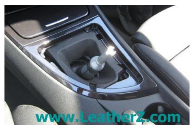
With the shift knob and boot removed, remove the trim by pulling up. There are a few clips holding it in place.
