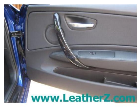
To remove the trim, begin at the bottom of the trim. I was able to remove by pulling the trim off, you may want to use an Interior Trim Tool to un-dock the connectors.
